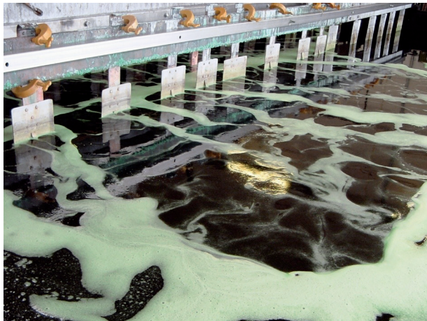
Fig. 28: View into an electropolishing bath used for electrolytic brightening of stainless steel. Reason for foam evolution is oxygen evolution at the anode and hydrogen evolution at the cathode
